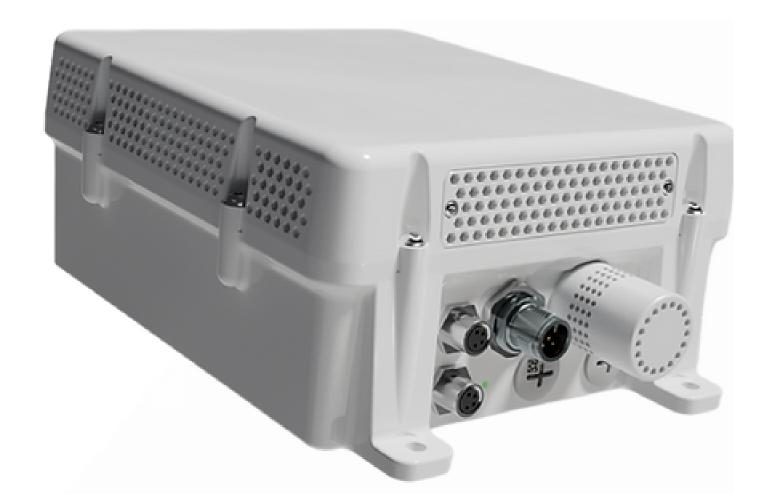
The sensors used are electrochemical gas sensors, designed to generate a current that is linear to the concentration of a target gas, by letting the gas interact with a working electrode. A critical challenge, however, is maintaining sensor accuracy over time, which is essential for reliable, longterm data collection.
